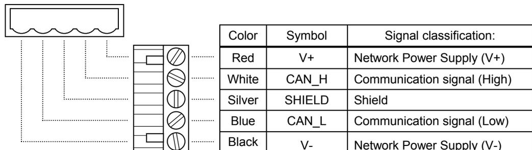
Size of connectable wire: 0.3 to 1.5mm<sup>2</sup> (AWG 22 to 16), Strip-off length: 7mm
