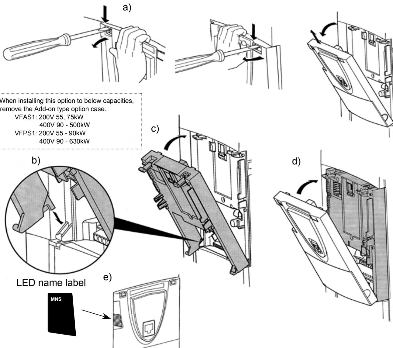
\* When installing this option to below capacities, remove the Add-on type option case.
