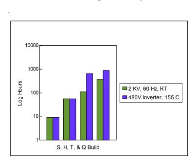
Note: No failures on Quadruple build in HV inverter after 2300 hours
