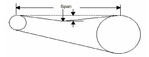
Apply force in the center of the span, at right angles to the belt with sufficient force to deflect the belt 1/64 th inch for each inch of span length. With properly tensioned belts, the force should fit into the ranges given. (The following information was compiled from several sources. The format provides the minimum and maximum values plus the average value shown in brackets.
