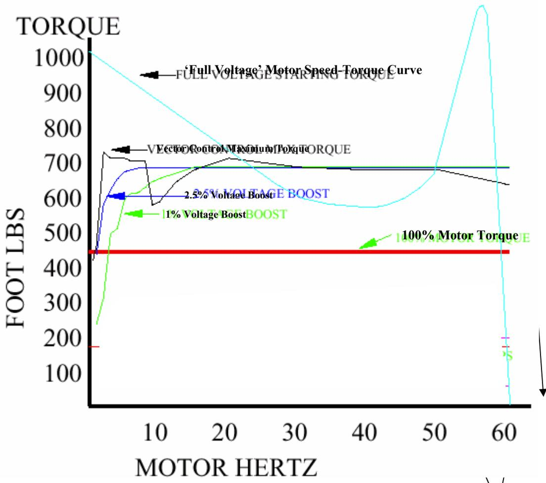
Because a motor and VFD system operates in the linear region of a motor speed-torque curve, the pull-up torque is higher than that of a typical 'full voltage' motor speed-torque curve. This being the case, a motor and VFD system can have improved starting capability in demanding applications, even when compared against an across the line start.
