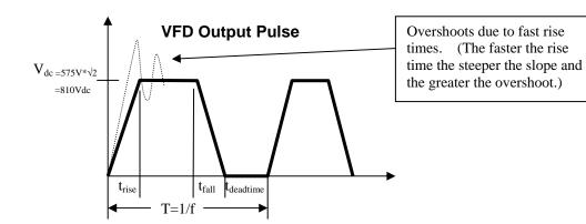
As rise times decrease (rate of rise or slope increases), the probability of a reflected wave increases with shorter and shorter cable lengths. This increases the voltage levels seen at the motor terminals. In theory, the voltage at the motor terminals can almost be doubled. (In actual installations, we have seen the voltage levels much higher, especially with multiple motors powered by one drive.)
